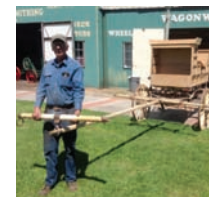
Completed pole system. The neck yoke at the front, tongue extending from the wagon, and double trees.
