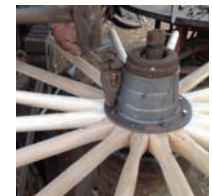
Riveting hickory spokes into a “Sarven” hub which were developed in the 1870s.
