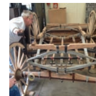
Paul Page adjusts brakes, used to slow it on downhills and hold it for loading/unloading.
